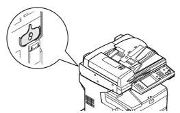
**4.** Fit plugs (2) in the scanner lock locations as shown.
